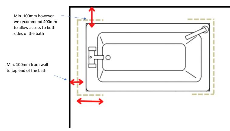
The floor directly under the bath located in the **yellow hatched area** must be sound, solid and even.
