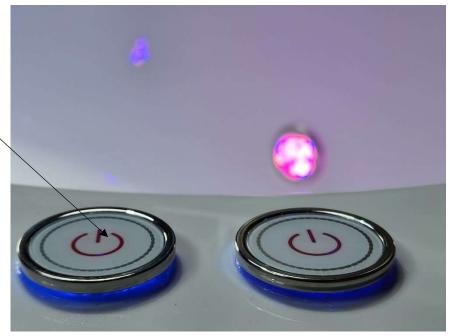
\*\* The buttons are touch sensitive, they do not require force to turn on and off – pressing these hard could cause damage \*\*
