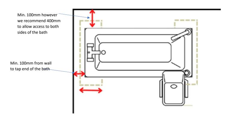
The floor directly under the bath located in the **yellow hatched area** must be sound, solid and even.
